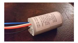
CONNECTION: Red= Phase White=Phase Blue=Phase Black=Neutral Dimensions Length 75 mm Diameter 44 mm Stud M8
