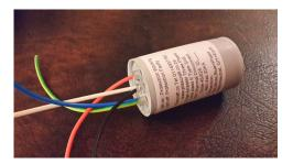
CONNECTION: Red= Phase White=Phase Blue=Phase Black=Neutral G/Y=Earth Dimensions Length 75 mm Diameter 44 mm Stud M8
